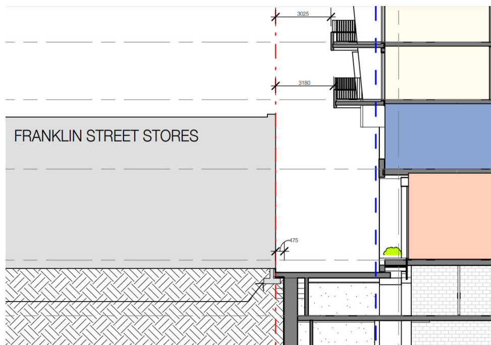
Figure 24: Cross section of Tower Two looking east showing the outer edge of the basement 475mm away from the southern face of the Franklin Street Stores. (Source: Tower Two architectural drawings).
