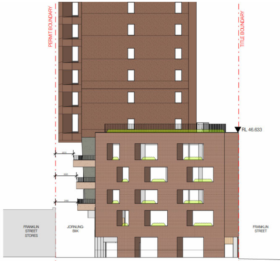
Figure 19: Cross section through Tower Two with the Franklin Street Stores at left. The wind canopy is not indicated, but the north face of the tower stops short of the parapet of the Stores. Mandatory setback above the podium under DPO11 is indicated at right. Because of this, the tower cannot be shifted back further to the south.
