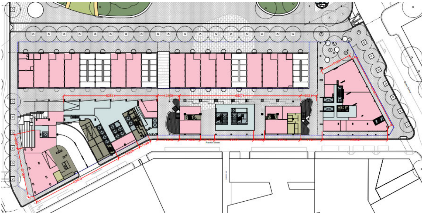
Figure 8: Plan showing the grid of the towers aligning with the grid of the Franklin Street Stores and the continuation of the laneway through the Franklin Street Stores and between Towers One and Two. (Source: OVGA Workshop 1 – Lendlease presentation)
