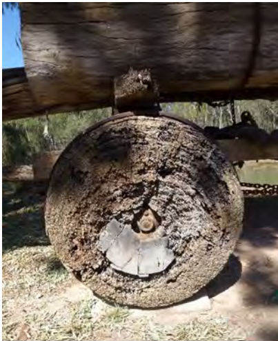
2021, Deteriorated timber on Log Buggy with modern insert
