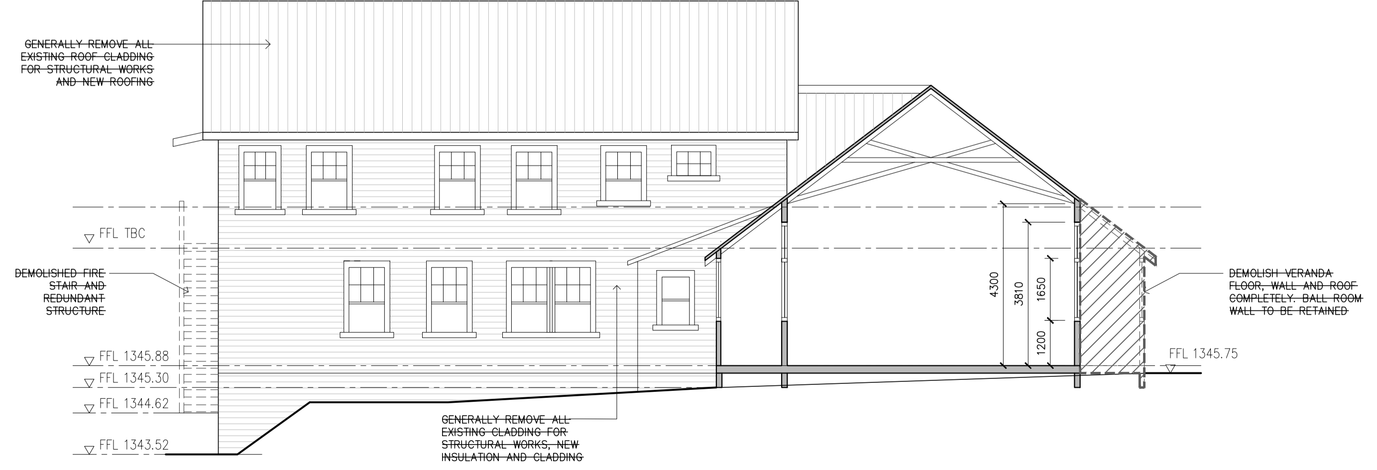
03 BUILDING 1A - EAST ELEVATION Scale 1:100 @ A1 / 1:200 @ A3
